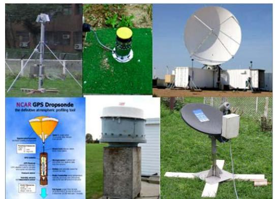
Rotate clockwise from upper left: Canada POSS, JW collision type disdrometer, US-NCAR S-band polarimetric (SPOL) radar system, Micro rain radar with wavelength of 1.25 cm, Korea vertically pointing rain profiler, and NCAR GPS dropsonde.
