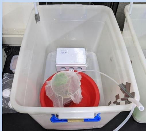
Figure 4. A simple system applied to study the influence of exhaust gas from automobiles on the development of aphid populations by the insect group
